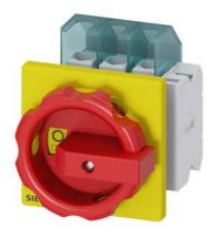
SENTRON, Switch disconnector 3LD, emergency switching-off switch, 3- pole, lu: 25 A, operating power / at AC-23 A 400 V: 9.5 kW, front-mounted, 1 NC, 1 NO, rotary operating mechanism, Red / yellow, 4-hole mounting of the handle
