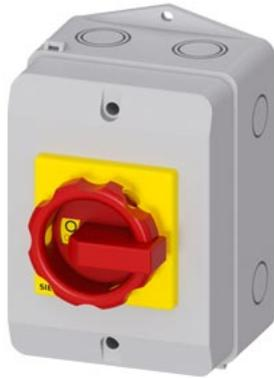
SETRON, Switch disconnecter 3LD, emergency switching-off switch, 4- pole, 16 A, operating power at AC-23 A at 400 V: 7.5 kW, molded-plastic encapsulation for metric cable gland, rotary operating mechanism, red/yellow
