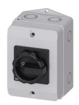
SENTRON, Switch disconnector 3LD, main switch, 3-pole, lu: 16 A, Operating power / at AC-23 A at 400 V:  $7.5~\mathrm{kW}$ , molded-plastic encapsulation for inch cable gland, rotary operating mechanism, black
