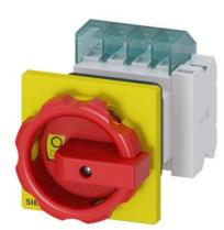
SENTRON, Switch disconnector 3LD, emergency switching-off switch, 3- pole, lu: 16 A, operating power / at AC-23 A 400 V: 7.5 kW, front-mounted, 1 NC, 1 NO, rotary operating mechanism, Red / yellow, Central mounting 22.5 mm of the handle
