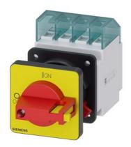
SENTRON, Switch disconnector 3LD, emergency switching-off switch, 4- pole, lu: 16 A, operating power / at AC-23 A 400 V: 7.5 kW, front-mounted, knob-operated mechanism, Red / yellow, central mounting 22.5 mm of the handle
