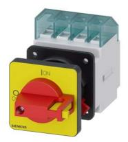
SENTRON, Switch disconnector 3LD, emergency switching-off switch, 3- pole, lu: 16 A, operating power / at AC-23 A 400 V: 7.5 kW, front-mounted, knob-operated mechanism, Red / yellow, central mounting 22.5 mm of the handle
