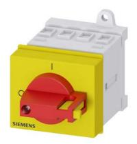
SENTRON, Switch disconnector 3LD, emergency switching-off switch, 4- pole, lu: 16 A, operating power / at AC-23 A 400 V: 7.5 kW, installation in distribution boards, knob-operated mechanism, Red / yellow, handle direct at the switch
