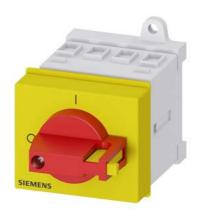
SENTRON, Switch disconnector 3LD, emergency switching-off switch, 3- pole, lu: 16 A, operating power / at AC-23 A 400 V: 7.5 kW, installation in distribution boards, knob-operated mechanism, Red / yellow, handle direct at the switch
