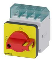
SENTRON, Switch disconnector 3LD, emergency switching-off switch, 4- pole, lu: 16 A, operating power / at AC-23 A 400 V: 7.5 kW, front-mounted, knob-operated mechanism, red/yellow, 4-hole mounting of the handle
