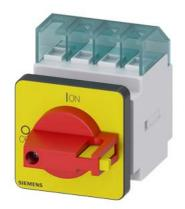
SENTRON, Switch disconnector 3LD, emergency switching-off switch, 3- pole, lu: 16 A, operating power / at AC-23 A 400 V: 7.5 kW, front-mounted, knob-operated mechanism, red/yellow, 4-hole mounting of the handle
