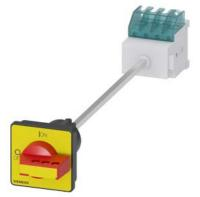
SENTRON, switch disconnector 3LD, EMERGENCY OFF switch, 4-pole, Iu: 16 A, Operating power / at AC-23 A at 400 V:  $7.5 \, \text{kW}$ , floor mounting with door coupling, defeatable knob-operated mechanism, red/yellow, 4-hole mounting of the handle
