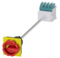
SENTRON, Switch disconnector 3LD, emergency switching-off switch, 4- pole, lu: 16 A, operating power / at AC-23 A 400 V: 7.5 kW, floor mounting with door coupling, rotary operating mechanism, Red / yellow, 4-hole mounting of the handle
