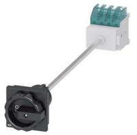
SENTRON, Switch disconnector 3LD, main switch, 3-pole, lu: 16 A, Operating power / at AC-23 A at 400 V: 7.5 kW, floor mounting with door coupling, rotary operating mechanism, black, 4-hole mounting of the handle
