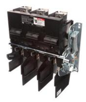
SIEMENS LOW VOLTAGE MCS SWITCH DISCONNECT (MOTOR CONTROL DISCONNECT). UL LISTED AND CSA CERTIFIED SWITCH. RATED 600V (200A). SPECIAL FEATURES: RIGHT HANDLE OPERATOR, FIELD INSTALLABLE AUXILIARY CONTACTS, FLANGE MOUNTED HANDLES.
