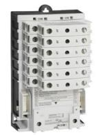
Electrically held lighting contactor, (convertible to mech. held), Amp rating 30A (tungsten 20A), 8 N.C. / 4 N.O. poles, 200-208V 60Hz coil, Non-combination type, Enclosure NEMA type (open), No enclosure
