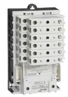
Electrically held lighting contactor, (convertible to mech. held), Amp rating 30A (tungsten 20A), 7 N.C. / 0 N.O. poles, 24V 60Hz / 20V 50Hz coil, Non-combination type, Enclosure NEMA type (open), No enclosure
