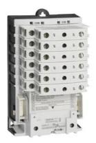
Electrically held lighting contactor, (convertible to mech. held), Amp rating 30A (tungsten 20A), 6 N.C. / 6 N.O. poles, 200-208V 60Hz coil, Non-combination type, Enclosure NEMA type (open), No enclosure
