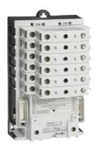
Electrically held lighting contactor, (convertible to mech. held), Amp rating 30A (tungsten 20A), 3 N.C. / 8 N.O. poles, 460-480V 60Hz/440V 50Hz coil, Noncombination type, Enclosure NEMA type (open), No enclosure
