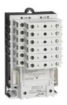
Electrically held lighting contactor, (convertible to mech. held), Amp rating 30A (tungsten 20A), 3 N.C. / 0 N.O. poles, 230-240V 60Hz/220V 50Hz coil, Noncombination type, Enclosure NEMA type (open), No enclosure
