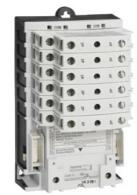
Electrically held lighting contactor, (convertible to mech. held), Amp rating 30A (tungsten 20A), 2 N.C. / 7 N.O. poles, 200-208V 60Hz coil, Non-combination type, Enclosure NEMA type (open), No enclosure
