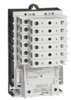
Electrically held lighting contactor, (convertible to mech. held), Amp rating 30A (tungsten 20A), 2 N.C. / 4 N.O. poles, 200-208V 60Hz coil, Non-combination type, Enclosure NEMA type (open), No enclosure
