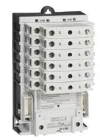
Electrically held lighting contactor, (convertible to mech. held), Amp rating 30A (tungsten 20A), 1 N.C. / 10 N.O. poles, 575-600V 60Hz/550V 50Hz coil, Non-combination type, Enclosure NEMA type (open), No enclosure
