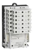
Electrically held lighting contactor, (convertible to mech. held), Amp rating 30A (tungsten 20A), 1 N.C. / 8 N.O. poles, 575-600V 60Hz/550V 50Hz coil, Noncombination type, Enclosure NEMA type (open), No enclosure
