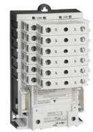
Electrically held lighting contactor, (convertible to mech. held), Amp rating 30A (tungsten 20A), 1 N.C. / 3 N.O. poles, 200-208V 60Hz coil, Non-combination type, Enclosure NEMA type (open), No enclosure
