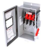
Siemens Low Voltage Circuit Protection Heavy Duty Safety Switches. Type: ENCLOSED, SAFETY SWITCH Std: UL V. Rating: 600V A. Rating: 200A Wattage: 2W No. Of Poles: 3P F. Rating: 60Hz Action: SINGLE THROW Material: 304SS Enclosure: TYPE 12. 2-3 point mounting holes. Insulation: YES O. Cycles: 8000 O. Temperature: (-20F-120F) AMBIENT TEMPERATURE Environmental Conditions: INDUSTRIAL
