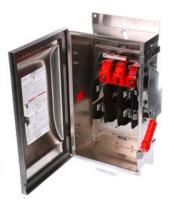
Siemens Low Voltage Circuit Protection Heavy Duty Safety Switches. Type: ENCLOSED, SAFETY SWITCH Std: UL V. Rating: 240V A. Rating: 200A Wattage: 3W No. Of Poles: 3P F. Rating: 60Hz Action: SINGLE THROW Material: SS Enclosure: TYPE 4X. 2-3 point mounting holes. Insulation: YES O. Cycles: 8000 O. Temperature: (-20F-120F) AMBIENT TEMPERATURE Environmental Conditions: INDUSTRIAL CORROSIVE RESISTANCE
