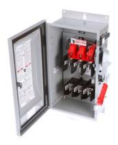
Siemens Low Voltage Circuit Protection Heavy Duty Safety Switches. Type: ENCLOSED, SAFETY SWITCH Std: UL V. Rating: 240V A. Rating: 200A Wattage: 3W No. Of Poles: 3P F. Rating: 60Hz Action: SINGLE THROW Material: 304SS Enclosure: TYPE 12. 2-3 point mounting holes. Insulation: YES O. Cycles: 8000 O. Temperature: (-20F-120F) AMBIENT TEMPERATURE Environmental Conditions: INDLISTRIAL
