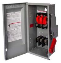
Siemens Low Voltage Circuit Protection Heavy Duty Safety Switches. Type: ENCLOSED, SAFETY SWITCH Std: UL V. Rating: 240V A. Rating: 100A Wattage: 4W No. Of Poles: 3P F. Rating: 60Hz Action: SINGLE THROW Material: 304SS Enclosure: TYPE 3R. 2-3 point mounting holes. O. Cycles: 10000 O. Temperature: (-20F-120F) AMBIENT TEMPERATURE Environmental Conditions: OUTDOOR
