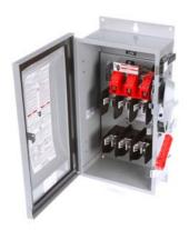
Siemens Low Voltage Circuit Protection Heavy Duty Safety Switches. Type: ENCLOSED, SAFETY SWITCH Std: UL V. Rating: 240V A. Rating: 60A Wattage: 3W No. Of Poles: 3P F. Rating: 60Hz Action: SINGLE THROW Material: 304SS Enclosure: TYPE 12. 2-3 point mounting holes. Insulation: YES O. Cycles: 10000 O. Temperature: (-20F-120F) AMBIENT TEMPERATURE Environmental Conditions: INDUSTRIAL
