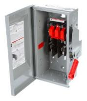
Siemens Low Voltage Circuit Protection Heavy Duty Safety Switch. 1-Pole 2-Wire and positive and negative ground Fused in a type 3R enclosure (outdoor). Rated 1000VDC (200A). Special features: photovoltaic rated, 10000 AIC disconnect.
