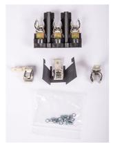
SIEMENS LOW VOLTAGE MCS SWITCH DISCONNECT ACCESSORY. J CLASS FUSE KIT FOR MCS SWITCH. RATED 600V (30A). WIRE RANGE: NO.14 - NO.4 AWG (CU/AL). INCLUDES LOAD BASE PLUS LINE AND LOAD FUSE CLIPS.
