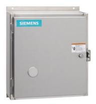
Mechanically held lighting contactor, Contactor amp rating 20Amp 0NC  $\_$  3NO poles, 265-277V 50/60HZ coil, Non-combination type, Encl NEMA type 4X 304 S-steel Water/dust tight noncorrosive
