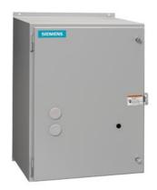
Mechanically held Lighting contactor Contactor amp rating 200Amp 0 NC / 3 NO poles 208VAC 60HZ coil Non-combination type Enclosure NEMA type 12 Dust/drip proof for indoors
