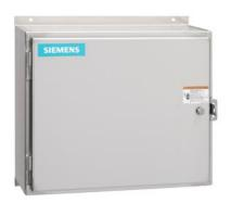
Mechanically held lighting contactor, Contactor amp rating 60Amp 0NC  $\_$  8NO poles, 220VAC 50HZ / 240VAC 60HZ coil Non-combination type, Enclosure NEMA type 12, Dust/drip proof for indoors
