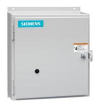
Mechanically held Lighting contactor Contactor amp rating 60Amp 0 NC / 4 NO poles 208VAC 60HZ coil Non-combination type Enclosure NEMA type 12 Dust/drip proof for indoors
