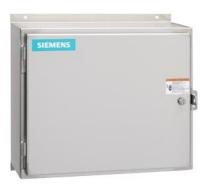
Mechanically held lighting contactor, Contactor amp rating 30A, 0 N.C. / 10 N.O. poles, 277VAC 60HZ coil, Non-combination type, Enclosure NEMA type 12, Dust/drip proof for indoors
