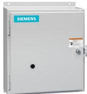
Mechanically held lighting contactor, Contactor amp rating 20A, 0 N.C. / 8 N.O. poles, Non-combination type, Enclosure NEMA type 12, Dust/drip proof for indoors
