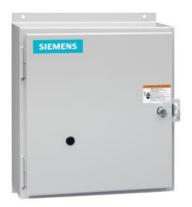
Mechanically held lighting contactor, Contactor amp rating 20A, 0 N.C. / 6 N.O. poles, Non-combination type, Enclosure NEMA type 12, Dust/drip proof for indoors
