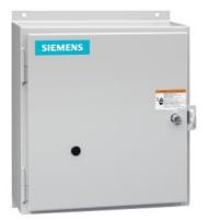
Mechanically held lighting contactor, Contactor amp rating 20A, 0 N.C. / 3 N.O. poles, Non-combination type, Enclosure NEMA type 12, Dust/drip proof for indoors
