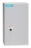
Mechanically held lighting contactor, Contactor amp rating 200A, 0 N.C. / 4 N.O. poles, 208VAC 60HZ coil, Non-combination type, Enclosure NEMA type 1, Indoor general purpose use
