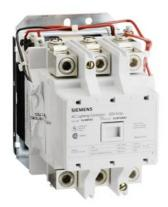
Mechanically held lighting contactor, Contactor amp rating 200A, 0 N.C. / 3 N.O. poles, 208VAC 60HZ coil, Non-combination type, Enclosure NEMA type (open), No enclosure
