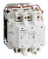
Mechanically held lighting contactor, Contactor amp rating 200A, 0 N.C. / 3 N.O. poles, 24VAC 60HZ coil, Non-combination type, Enclosure NEMA type (open), No enclosure
