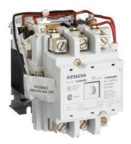
Mechanically held lighting contactor, Contactor amp rating 60A, 0 N.C. / 3 N.O. poles, 440VAC 50HZ/480VAC 60HZ coil, Non-combination type, Enclosure NEMA type (open), No enclosure
