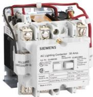
Mechanically held lighting contactor, Contactor amp rating 30A, 0 N.C. / 3 N.O. poles, 208VAC 60HZ coil, Non-combination type, Enclosure NEMA type (open), No enclosure
