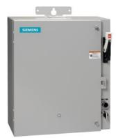
Pump control panel, Size 6, Three phase full voltage, Solid-state overload relay, OLR amp range 160-630A, 220-240V 50-60Hz/DC coil, Standard type contactor, 400A circuit breaker, HOA Sel Sw. <(>&<)> Start P.B., Enclosure NEMA type 3/3R, Weather proof outdoor use
