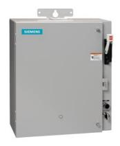
Pump control panel, Size 5, Three phase full voltage, Solid-state overload relay, OLR amp range 55-250A, 220-240V 50-60Hz/DC coil, Standard type contactor, 250A circuit breaker, HOA Sel Sw. <(>&<)> Start P.B., Enclosure NEMA type 3/3R, Weather proof outdoor use
