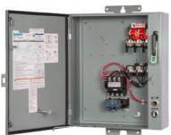
Pump control panel, Size 2 1/2, Three phase full voltage, Solid-state overload relay, OLR amp range 25-100A, 110-120/220-240VAC 60Hz coil, Standard type contactor, 60A fusible disconnect, 60A/250V fuse clip, HOA Sel Sw. <(>&<)> Start P.B., Enclosure NEMA type 3/3R, Weather proof outdoor use
