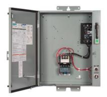
Pump control panel, Size 1, Three phase full voltage, Solid-state overload relay, OLR amp range 5.5-22A, 190-220/220-240V 50/60Hz coil, Standard type contactor, 25A circuit breaker, HOA Sel Sw. <(>&<)> Start P.B., Enclosure NEMA type 3/3R, Weather proof outdoor use
