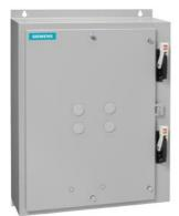
Duplex starter w/ alternator, Size 2 1/2, Three phase full voltage, Solid-state overload relay, OLR amp range 25-100A, 110V 50Hz / 120V 60Hz coil, Combination type, Two 100A circuit breakers, Enclosure NEMA type 12, Dust/drip proof for indoors
