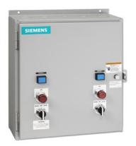
Duplex starter w/ alternator, Size 0, Three phase full voltage, Solid-state overload relay, OLR amp range 0.75-3.4A, 110V 50Hz / 120V 60Hz coil, Non-combination type, Enc NEMA type 4 painted steel, Water/dust tight for outdoors
